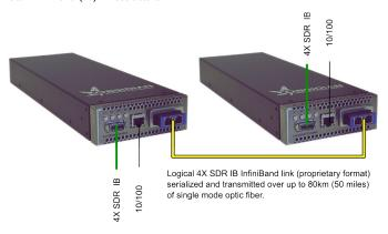
The Longbow C100 series devices report as two-port IB switches to the subnet manager – the IB fabrics at the two end-point locations unify into a single subnet.
