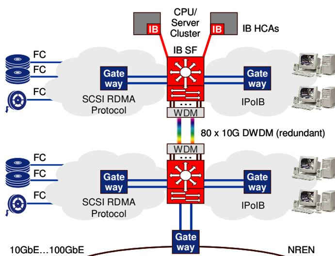
Fig. 1. Metro and national research and educational network. IB SF: InfiniBand Switch Fabric. HCA: Host Channel Adaptor.
