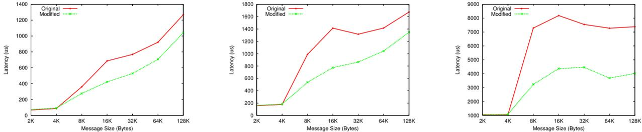
Figure 7. MPI broadcast latency over IB WAN: (a) 10us delay (b) 100us delay (c) 1000us delay
