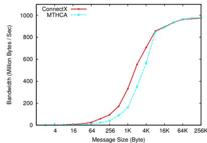
Figure 10. Verbs level RC Bandwidth with 1ms Network Delay
