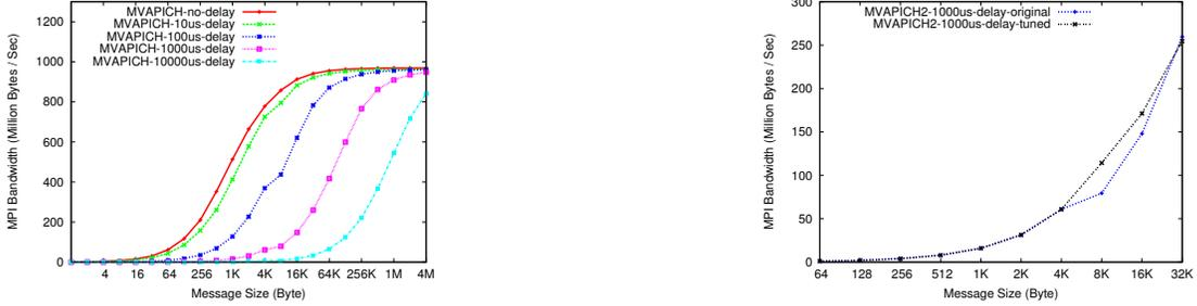
Figure 5. MPI-level throughput using MVAPICH2: (a) Original (b) Varying thresholds
